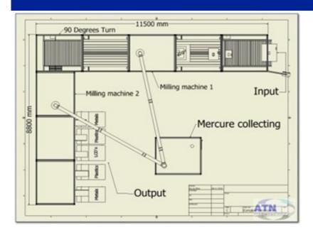
For instance, flat screen monitor and CRT recycling is increasingly becoming an issue. Collecting the mercury and other harmful materials in an environmentally friendly way and separating the materials has to be done in a machine, in order to avoid polluting the operators' work area. A capacity of up to 50 per hour is possible.
