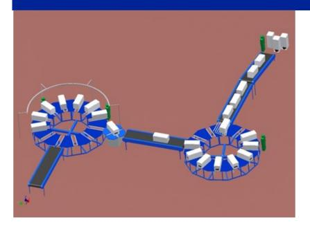
From a small conveyor up to a complete carousel system for processing more than 150 refrigerators per hour. Everything you need to make your refrigerator recycling as efficient as possible. Combined with our degassing machines, it is even possible to create semi-automatic degassing systems. Custom-made logistics systems for stage one degassing units and all kinds of systems for the manual and automatic disassembly of CRT-televisions and flat screens are also available.
